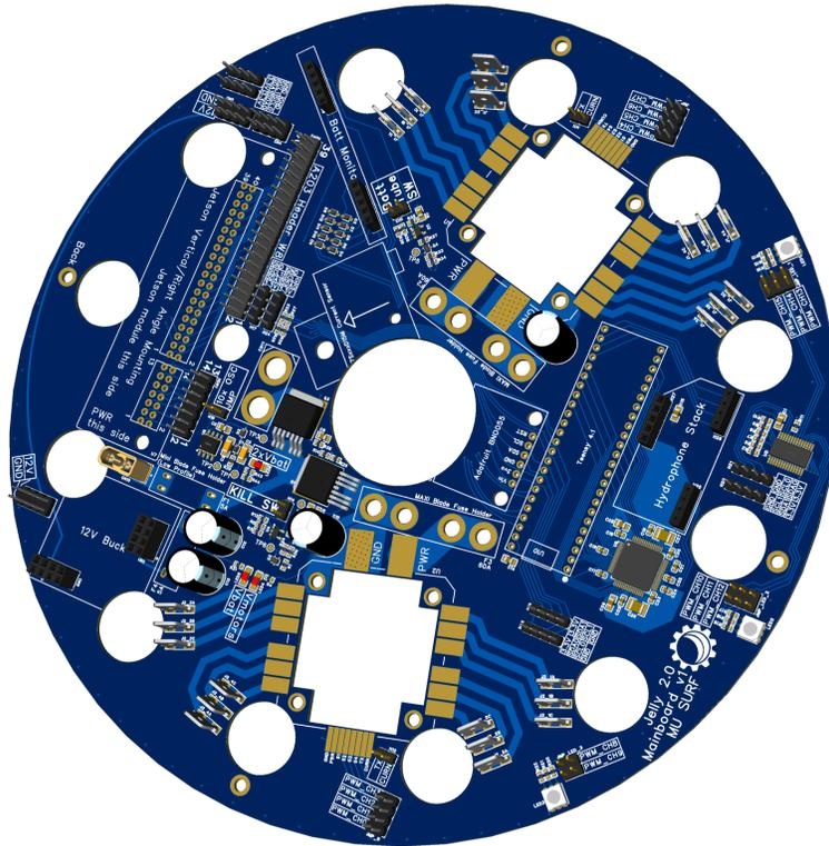
Fig. 5: Power distribution PCB (also referenced as “motherboard”)
