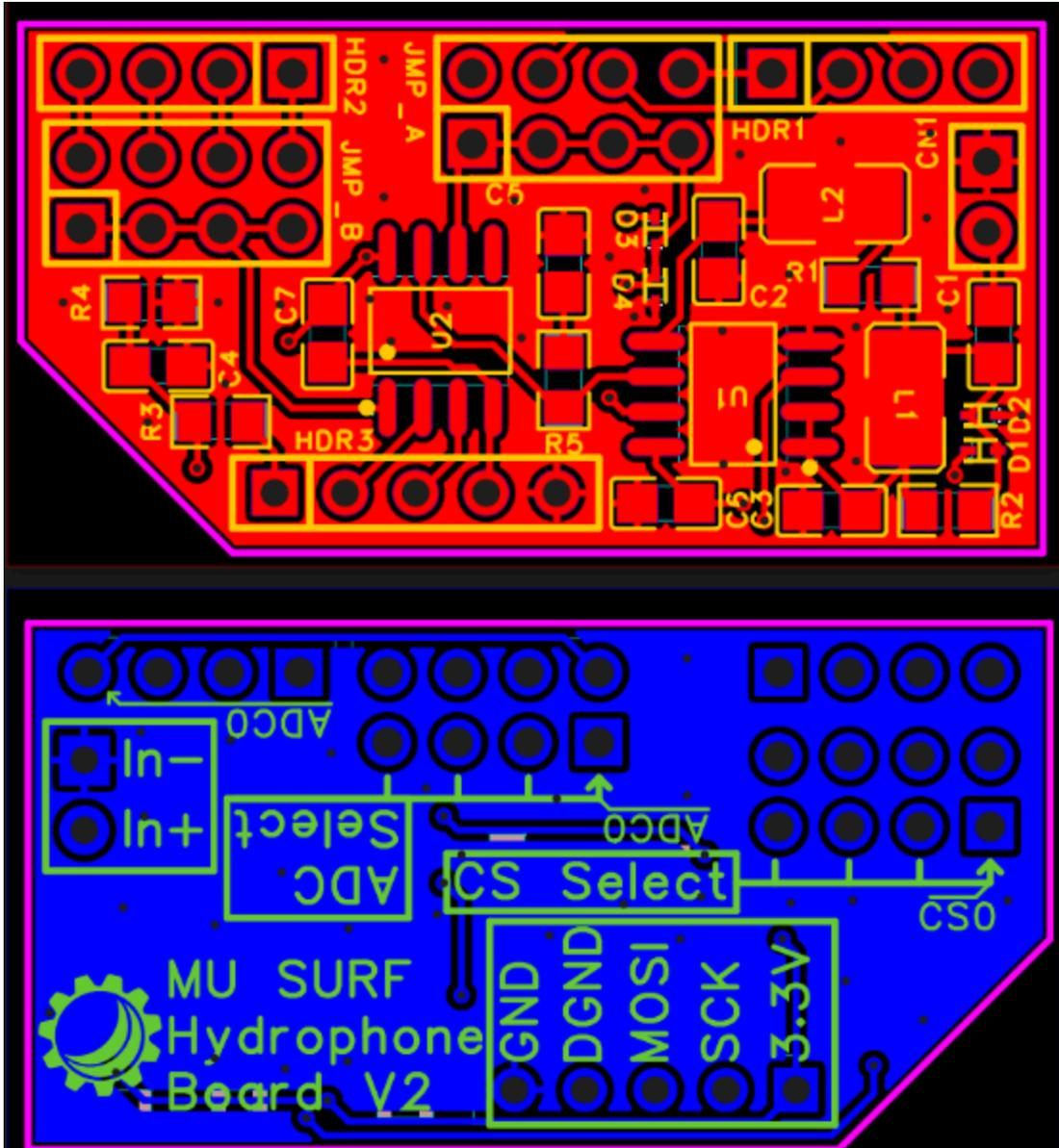
Fig. 8: Hydrophone stack PCB
