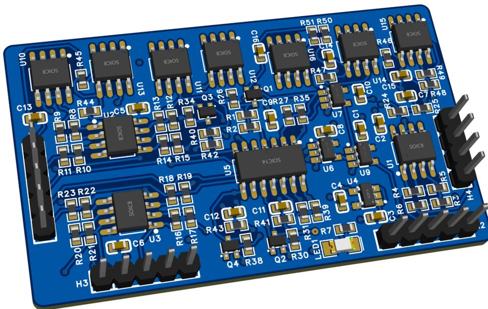
Fig. 6: Battery monitor PCB
