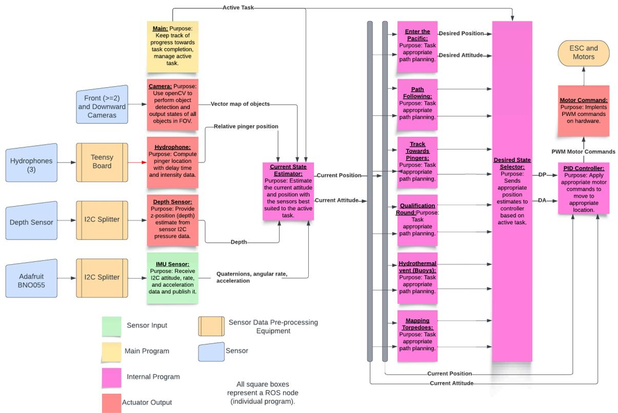
**Fig. 4: System engineering design of submarine operation**
