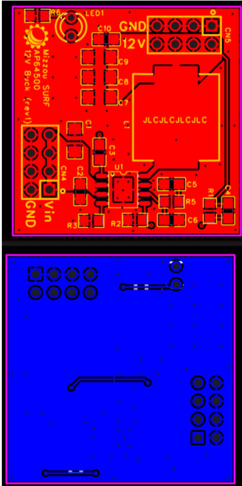
Fig. 7: Buck converter PCB
